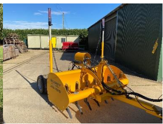
EG2 – Dual Grade kit Fitted to towed Laser Grader
