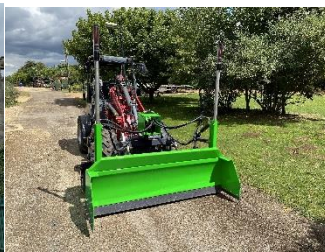
EG2 – Dual Grade Kit Fitted to front loader
